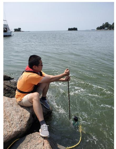
YAN USES A SIDE-LOOKING ADCP TO MEASURE THE INFLOWS AT A GUILFORD SALT MARSH INLET (PHOTO: KAY HOWARD-STROBEL)
